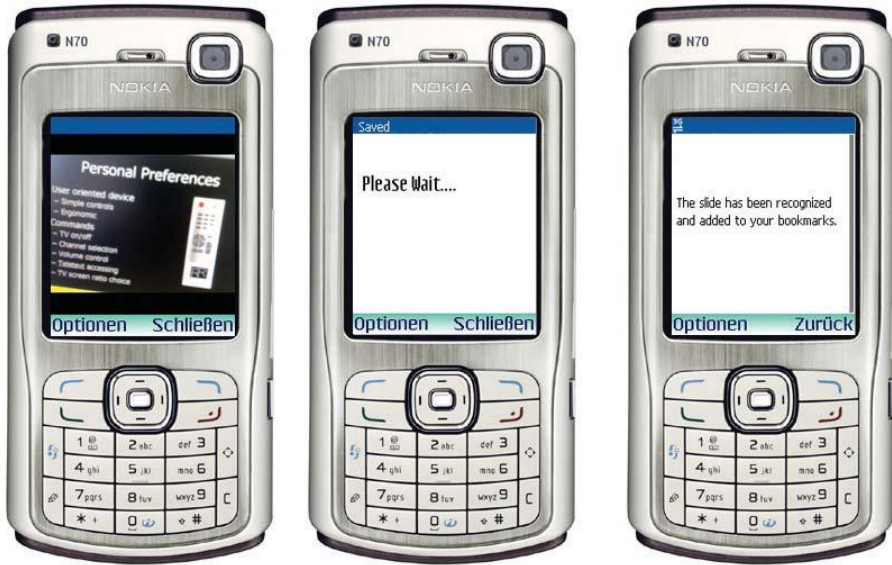
Fig. 1. The user "tags" a presented slide using our mobile application by taking a picture (left), which is automatically transmitted to the server and recognized (middle), a response is given in an automatically opened WAP browser (right).
