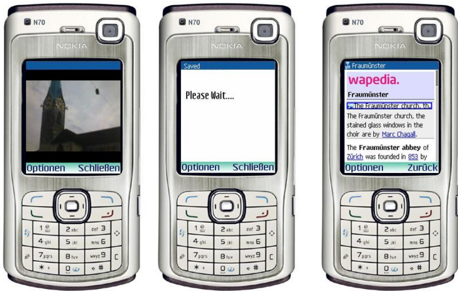
Fig. 4. Client software for the cityguide application: the user snaps a picture, waits a few seconds, and is redirected to the corresponding Wikipedia page
