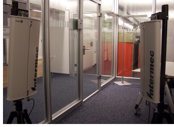
Fig. 3. UHF gate reader for inventory management
